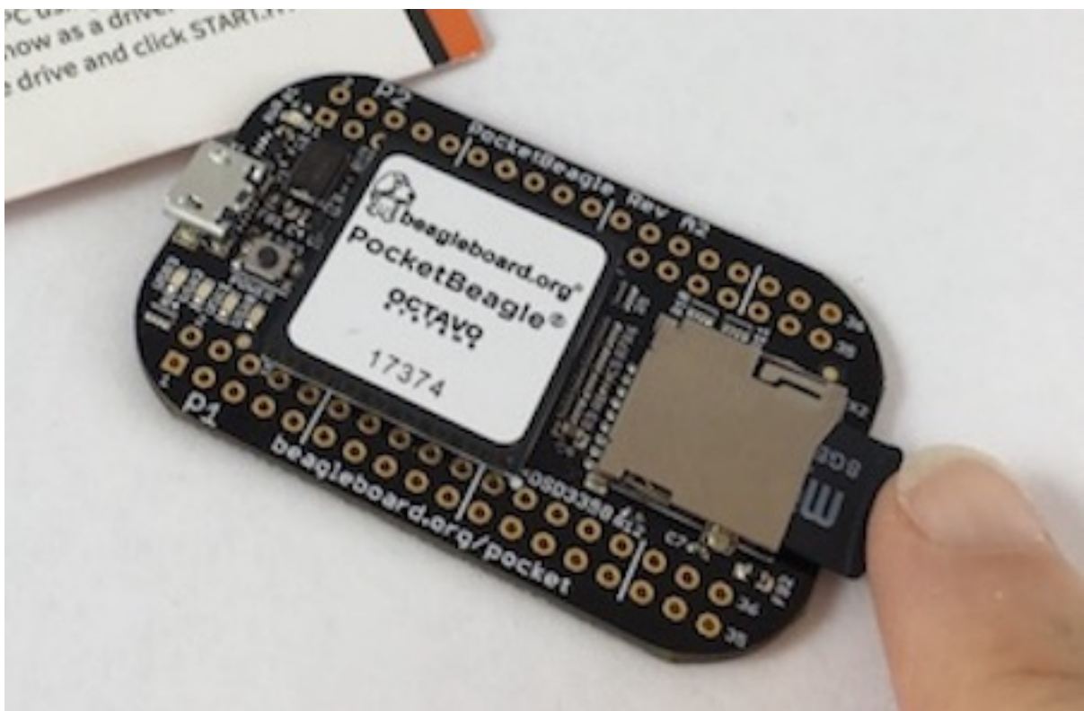
Fig. 3.10: Insert the microSD Card into PocketBeagle
