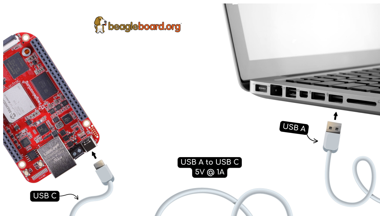
Fig. 2.2: BeagleV-Fire tethered connection
