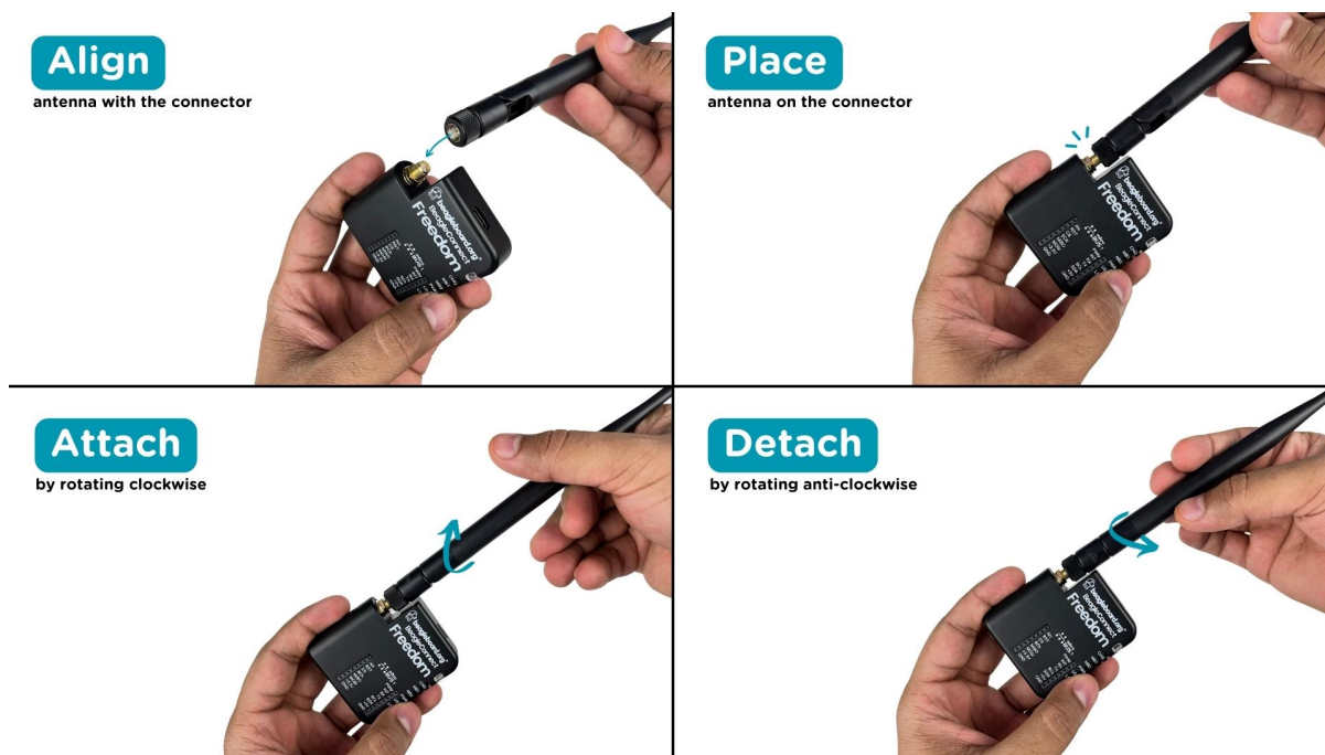
Fig. 2.2: Attaching antenna to BeagleConnect Freedom
